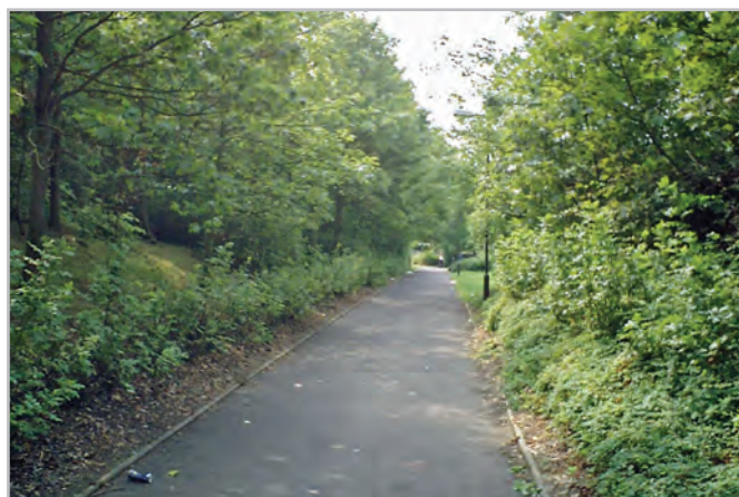
Segregated pedestrian and cycle routes provide no natural surveillance and should be omitted from schemes
