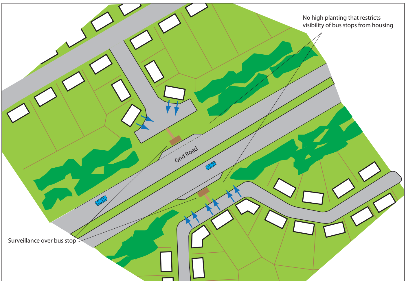
Two possible layouts to achieve safe pedestrian access to a bus stop
