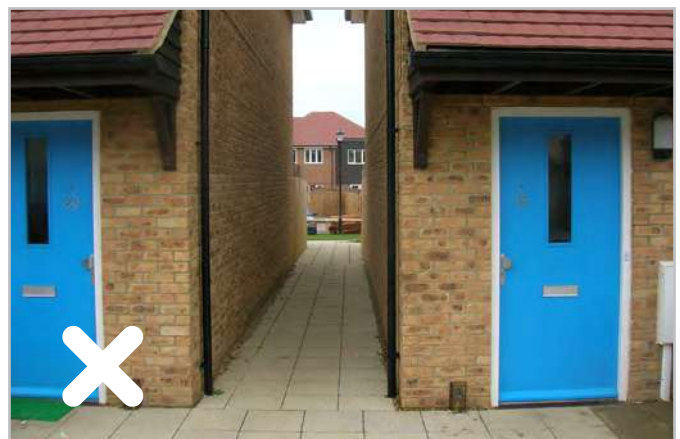
Only one entrance for vehicles/pedestrians is permitted. Unlocked alleyways will not be permitted
