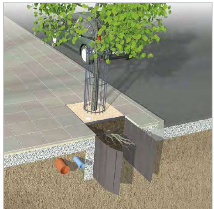
Root protection barrier detail
