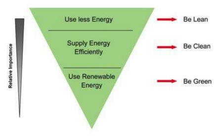
Figure 10 Energy Hierarchy (Source: BREEAM Passive design - Designing Buildings)
