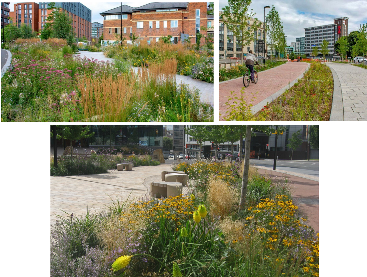
Figure 5 Images from recent Arup project in Sheffield. Aimed to renew urban realm with multi-functional SuDs incorporating spaces to move and dwell in. SuDs promoted drainage, biodiversity, climate adaptation, improved air quality and urban cooling. Image credits: Upper two images - Nigel Dunnett (2023); Lower image - Arup (2023).
