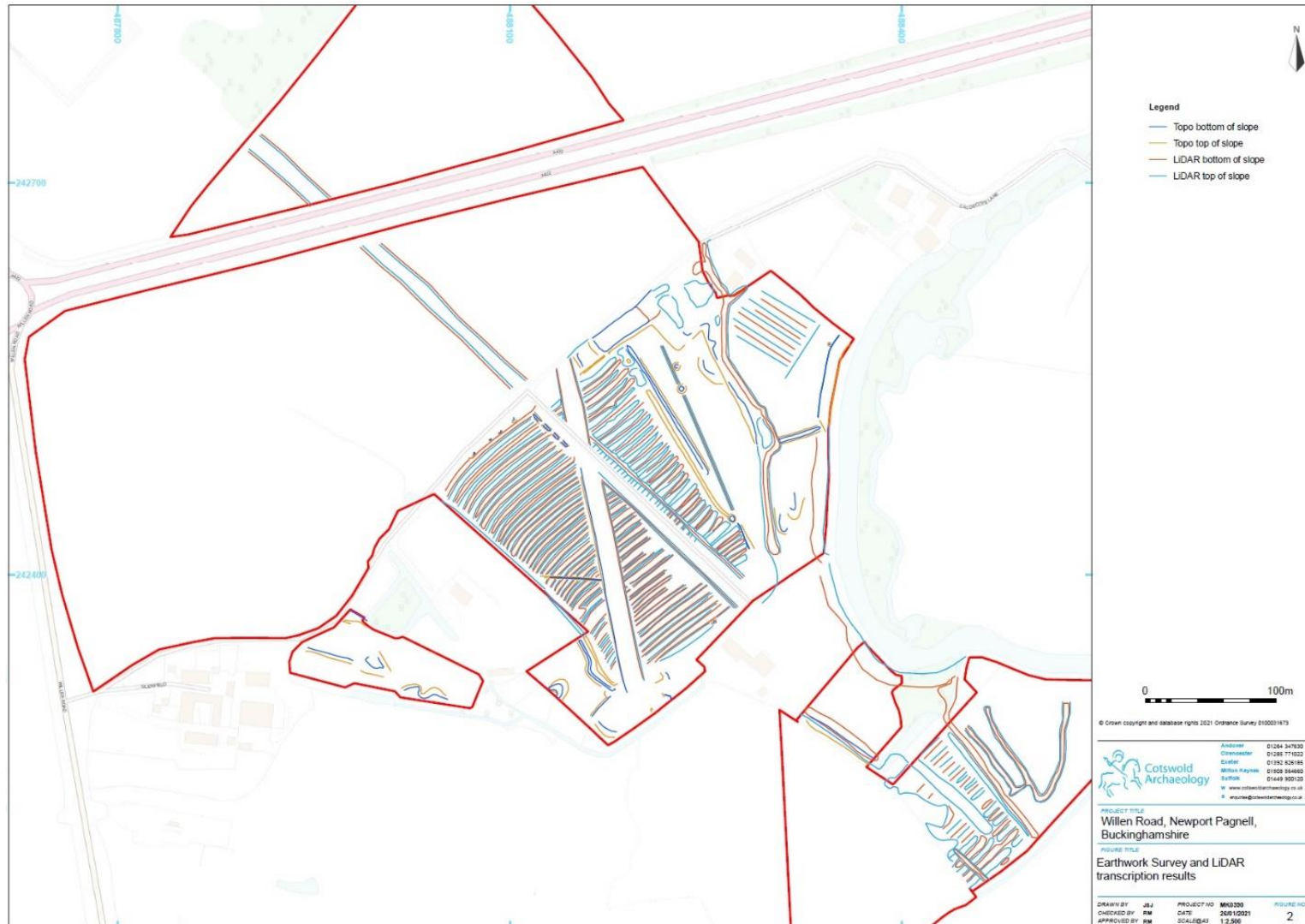
Figure 6.20: Interpretative earthwork survey drawing
