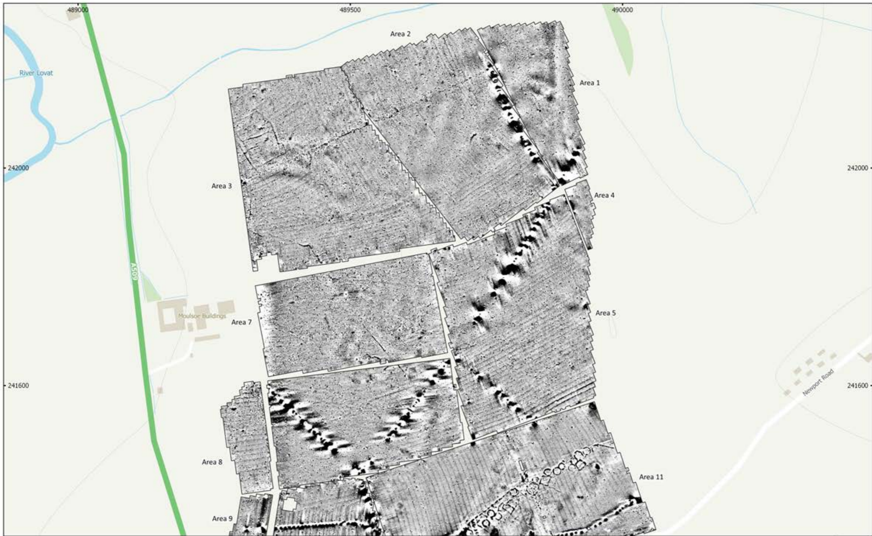
MSSP655 - Land East of Milton Keynes, Buckinghamshire Figure 3 - Magnetic Total Field (Lower Sensor) (Overview) (North) 1:4,000 @ A3 Copyright Magnitude Surveys Ltd 2020 Contains Ordnance Survey data © Crown Copyright and database right 2020
