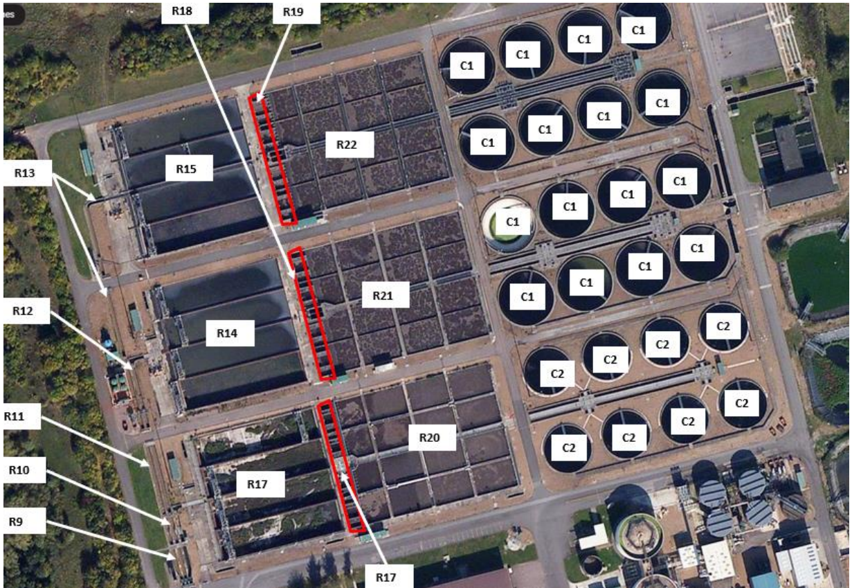
Figure 8: Cotton Valley WRC – Primary Settlement tanks, Storm Tanks & Activated Sludge Plant odour sources.
